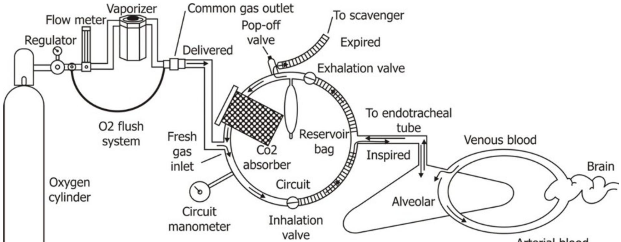
**Anesthesia delivery system showing the pathway traveled by anesthetic, from the vaporizer to the brain.**
